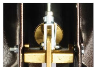
Fine tuner mechanism (if applicable)
