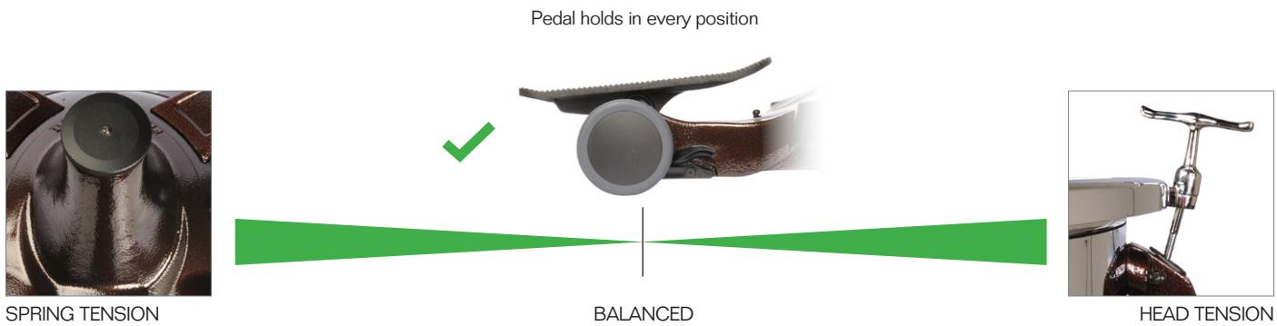
The balanced action pedal system functions correctly when the head tension and spring tension are in equilibrium. If the fundamental tone is not tensioned correctly, or the spring tension is too weak or strong compared to the correct fundamental tone, the pedal will not hold in place and the tone will change.
